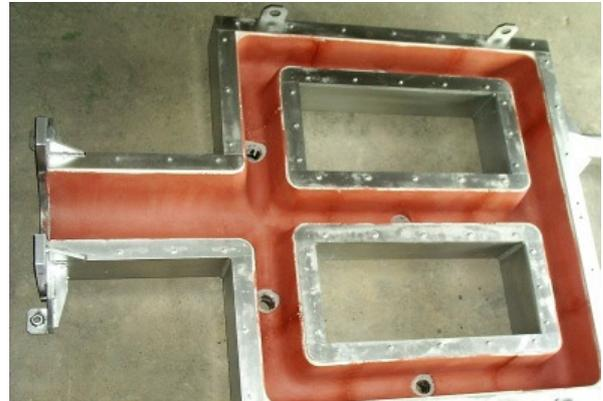
Precast launder assembly in fused silica material
