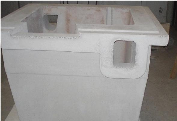
Precast liner for ALPUR degassing unit
